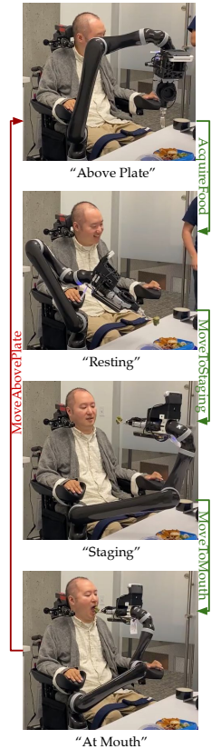
Figure 1.6: Key waypoints where the robot waits. “Above Plate,” “Resting,” and “Staging,” are fixed, whereas “At Mouth” depends on the perceived mouth location. Green arrows (right) shows progression when feeding the user, and red (left) when moving back for another bite.
