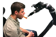
Figure 2.10: Bite transfer is the process of moving a bite of food to the user's mouth. Reprinted from [40].
