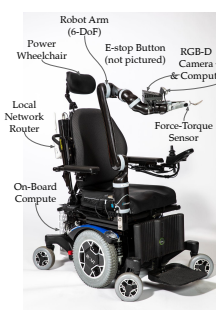
Figure 1.4: The robot-assisted feeding system consists of a wheelchair-mounted robot arm with an on-board RGB-D and force-torque sensor, router, and compute.
