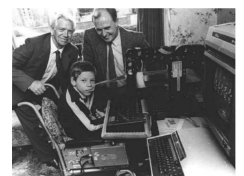
Figure 2.4: The Handy 1 was developed in 1987 to help a boy with cerebral palsy to independently eat. Reprinted from [127].
