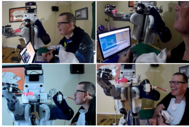
(a) A mobile manipulator robot-assisted feeding system feeding a user in their home. Reprinted from [236].
