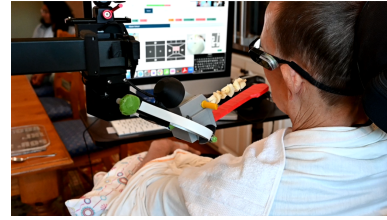
(c) A user teleoperates a mobile manipulator to feed himself in his home. Reprinted from [252].
