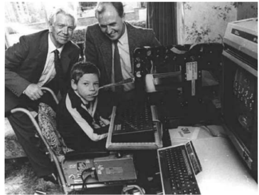
(d) The Handy 1 was developed in 1987 to help a boy with cerebral palsy to independently eat. Reprinted from [296].
