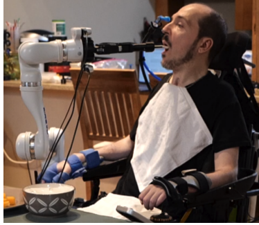
(b) A wheelchair-attached robot-assisted feeding system feeding a user in their home. Reprinted from [144].
